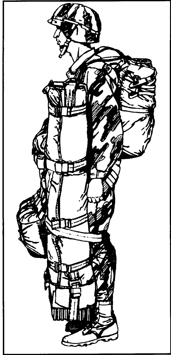
Figure 12-60. Lower tie-down tape routed around AT4JP.
