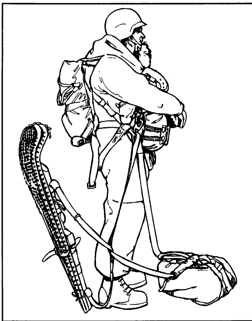
Figure 13-7. Lowering line assembly attached for a tandem load.
