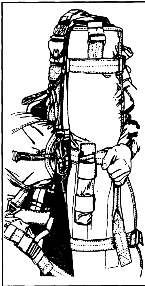
Figure 12-58. Attaching equipment to parachutist.
