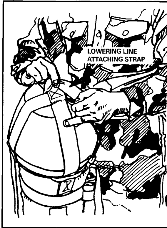
Figure 12-36. Lowering line attaching strap installed.
